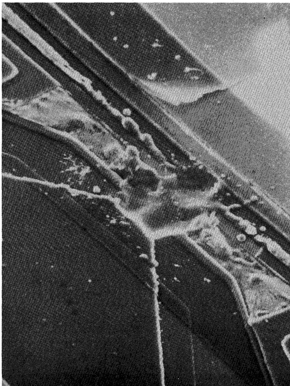
Fig. 9. Gate step failure; most dramatic example yet seen. Also shows peeled glassification overlay.
